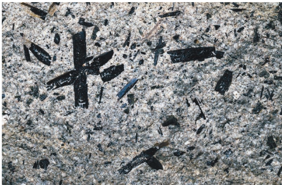
FIGURE 3.22 Amphibole crystals were among the first to crystallize in this “granitic” rock and therefore have well-developed crystal faces. The largest grain is about 3 cm long.
