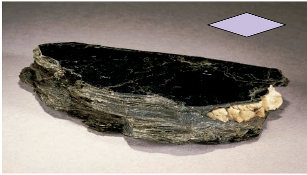
(A) One plane of cleavage in mica produces thin plates or sheets.
