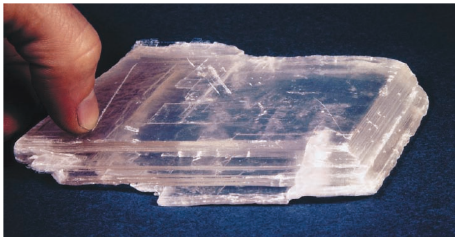
FIGURE 3.10 Hardness reflects the strength of the atomic bonds inside the mineral. Gypsum has a hardness of 2 on Mohs hardness scale. It is a very soft mineral and can easily be scratched with a fingernail.
